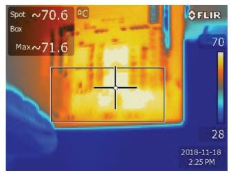
Fig. 19. Two-Phase ZIV Converter 35A Load Top Phase Thermal Image
