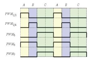
Fig. 2. Single-Phase ZIV Converter Gate Drive Diagram
