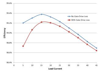
Fig. 22. Two-Phase ZIV Converter Efficiency Curve, No Cooling
