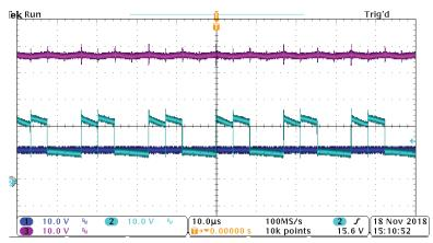
Fig. 15. Input Voltage, Node 1 Voltage, Output Voltage, 30A Load
