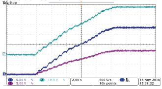
Fig. 21. Input Voltage, C<sub>f1</sub> and C<sub>f2</sub> Voltage Waveforms During Start-Up
