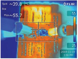
Fig. 26. Two-Phase ZIV Converter 45A Thermal Image, Fan Cooling
