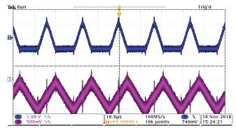
Fig. 18. Cf3 and Cf4 AC Ripple Voltage Waveforms, 30A Load
