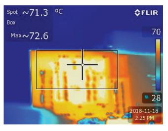
Fig. 20. Two-Phase ZIV Converter 35A Load Bottom Phase Thermal Image
