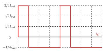
Fig. 5. Single-Phase ZIV Converter Input Capacitor Current
