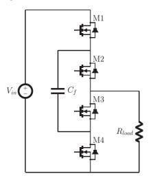
Fig. 7. Switched Capacitor "Building Block"
