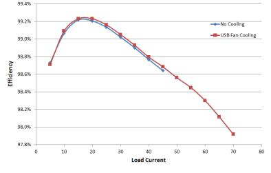
Fig. 25. Two-Phase ZIV Converter Efficiency, Gate Loss Included
