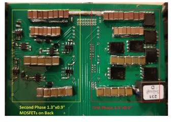
Fig. 14. Two-Phase ZIV Converter Prototype, Note that both phases are "mirrors" of each other
