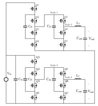
Fig. 3. Two-Phase ZIV Converter
