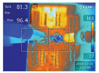
Fig. 27. Two-Phase ZIV Converter Full-Load 70A Thermal Image, Fan Cooling
