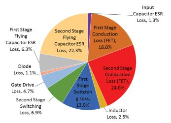
Fig. 13. Loss Breakdown for 45A Output Current
