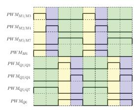
Fig. 4. Two-Phase ZIV Converter Gate Drive Diagram
