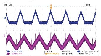
Fig. 17. Cf1 and Cf2 AC Ripple Voltage Waveforms, 30A Load
