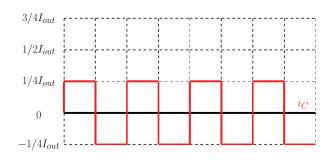
Fig. 6. Two-Phase ZIV Converter Input Capacitor Current
