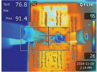
Fig. 23. Two-Phase ZIV Converter Full-Load 45A Thermal Image, No Cooling
